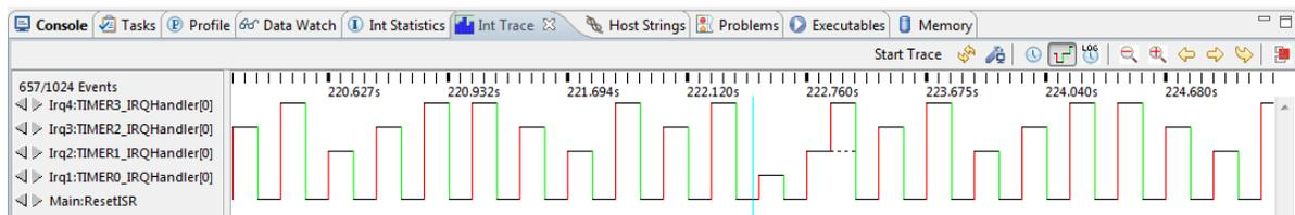
**Figure 5 - Interrupt Trace View**
